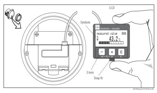
The VU331 LCD display can be removed to ease operation by simply pressing the snap-fit (see graphic above). It is connected to the device by means of a 500 mm (20") cable.
