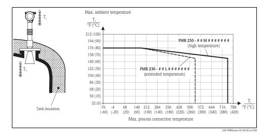
For process connection temperatures (T2) above  $80^{\circ}$ C (176°F), the allowed ambient temperature (T1) at the housing is reduced according to the above diagram.
