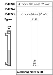
1) For media group A and B to use a Levelflex M with koax probe
